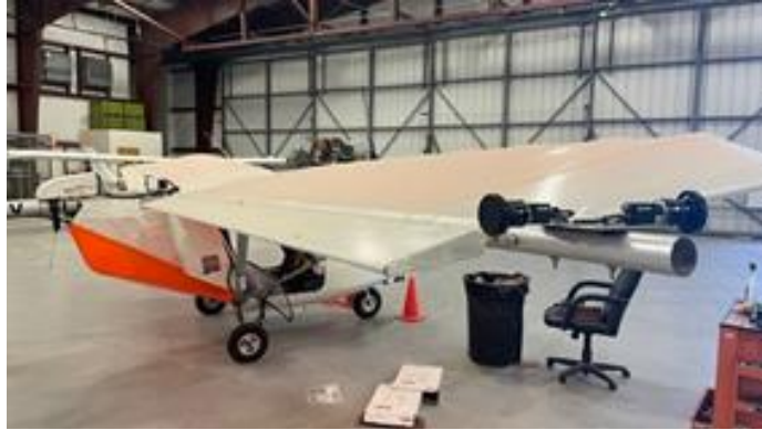
Figure 48. CasiaX cameras mounted on the right wing of ownship.
