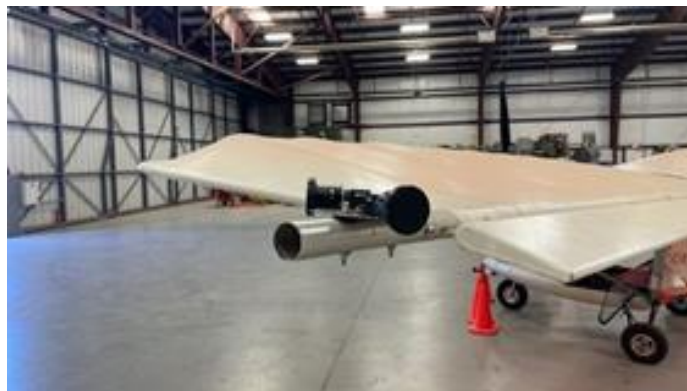
Figure 47. CasiaX cameras mounted on the left wing of ownship.
