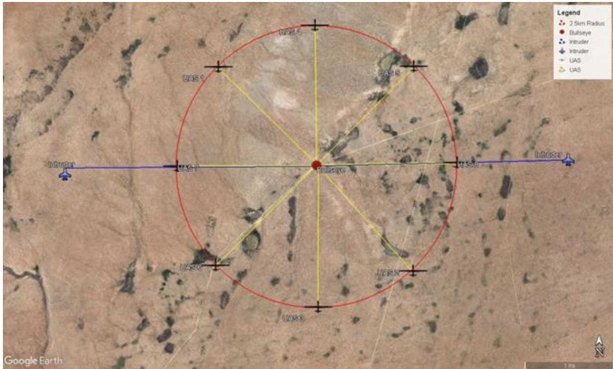
Figure 50. Configuration of horizontal encounters executed during the Fall 2021 NMSU campaign.
