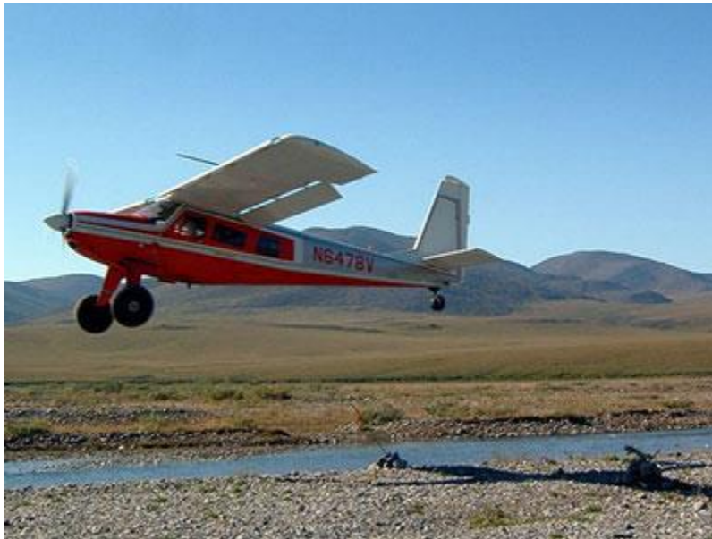
Figure 34. Helio Courier 295 CA used as an intruder during the June 2021 UAF campaign.
