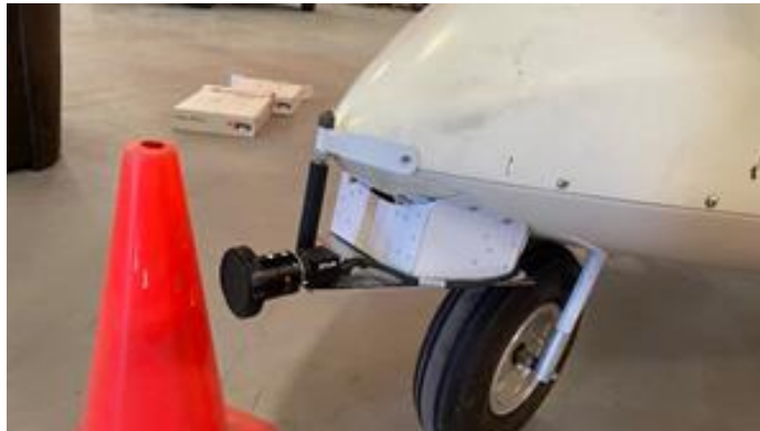
Figure 49. CasiaX camera mounted on the front of ownship.
