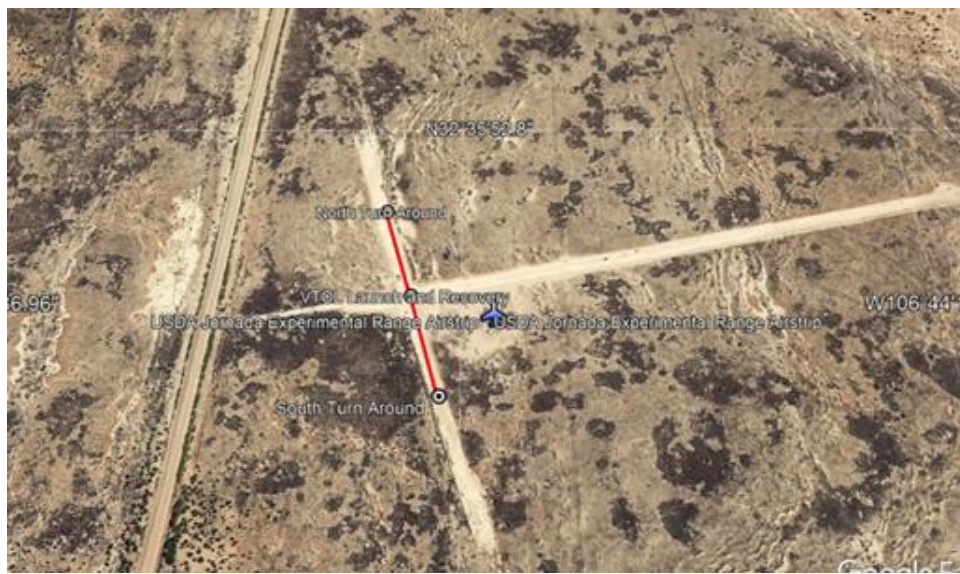
Figure 16. Example multi-copter UAS flight path. The fixed wing UAS path doubles this length and loops at the ends.
