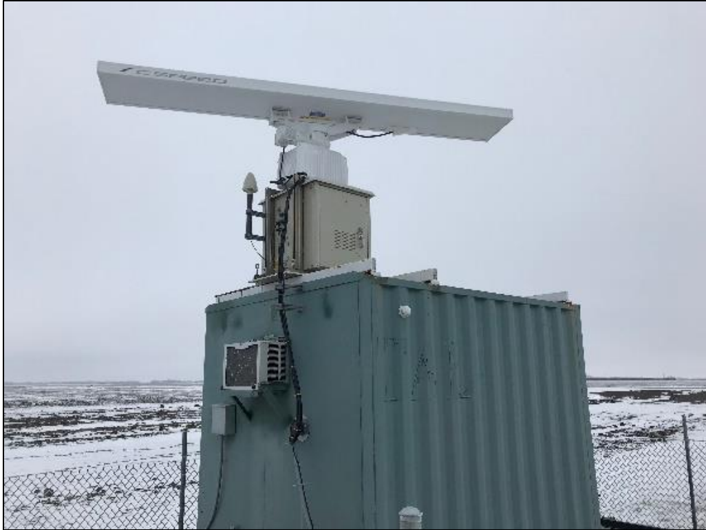
Figure 29. The C Speed Lightwave Radar utilized during the September 2020 UND campaign.
