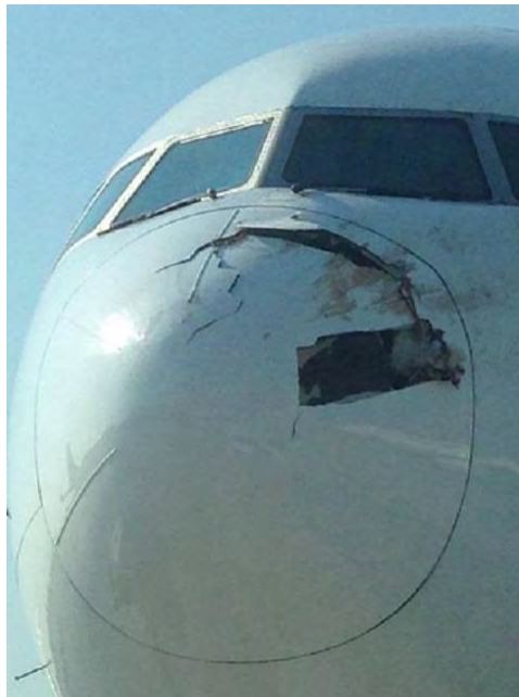
Figure 140. Boeing 777 with bird strike to radome (Chong, 2015).
